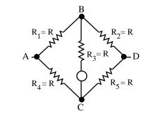
resistor between A and the point of interest). That means that the voltages at B and C will be equal. With no voltage difference between those points, there will be no current through that branch and this response is false. NOTE: If you re-sketch the circuit into the form shown, the observations made above are even easier to see.]
