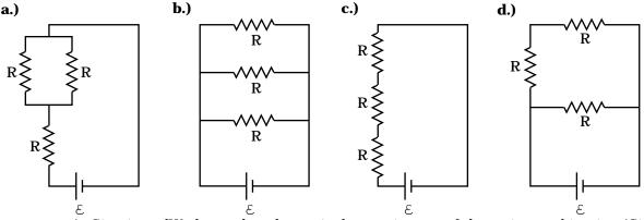
a.) Circuit a. [We know that the equivalent resistance of the series combination (Circuit c) will be the largest, and we know that the equivalent resistance of the parallel combination (Circuit b) will be the smallest. We can eliminate them. As for the other two, the equivalent
