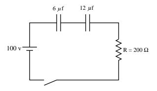
the power supply. That means that  $(100 \text{ volts}) = \frac{Q}{C_1} + \frac{Q}{C_2} = \frac{Q}{(6x10^{-6} \text{ farads})} + \frac{Q}{(12x10^{-6} \text{ farads})},$
